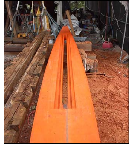
Final centerboard slot
