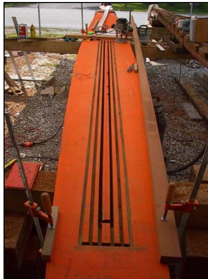
Cutting the centerboard trunk slot
