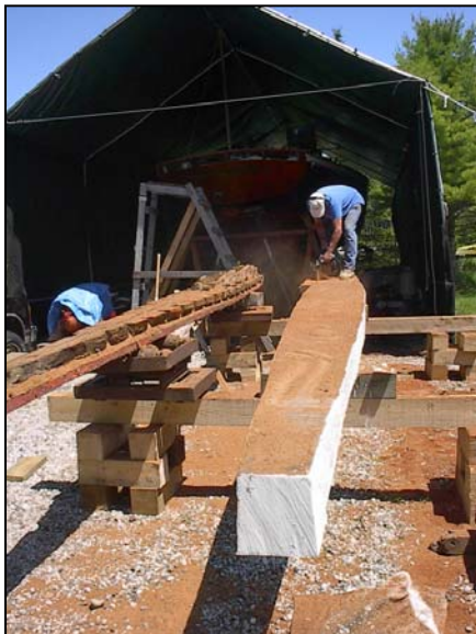
Roughing out the blank
