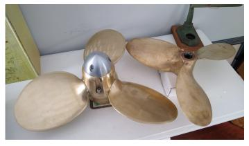
start with the prop. We really only looked at two very displacement. In our case, the corners of the sternpost in the aperture were square and needed to be Veriprop GP (grand performance). Again Malabar II rounded and faired back. This eliminated the haradmitted to having a 4 blade Veriprop GP and gaining monic vibration we had with the 4-107 (pressure waves reflecting back as the blade swings through the aperture).
