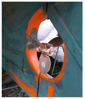
sions and other items settled on the D2-60. Again The prop must be sized to the aperture allowing suffieveryone has an opinion, so this is not a recommen- cient area around the tips and a laminar flow from the
